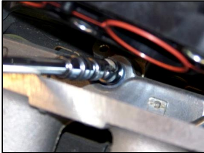
Figure 6: Remove Fuel Rail Mounting Nuts
