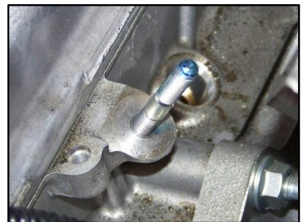
Figure 8: Remove Intake Manifold Studs
