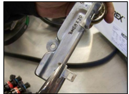
Figure 7: Removing Metal Tabs from Fuel Rail
