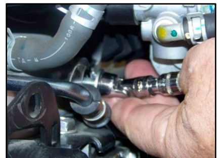
Figure 4: Unbolt Fuel Rail Bolt under Throttle Body
