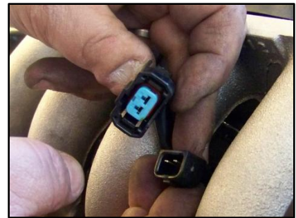
Figure 12: Injector Clips to Injector Leads
