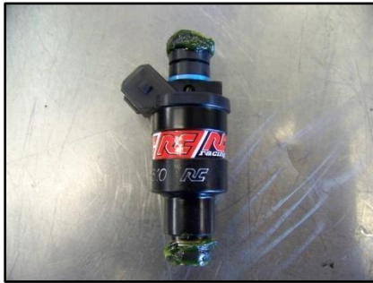
Figure 9: Properly Greased Injector
